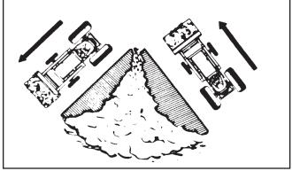
Sidecutting is a good technique for cutting down a big pile.
